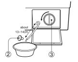
3. Remove any foreign material from the pump filter(3). After cleaning, turn the pump filter clockwise and insert the cap hose(2) to the original place. Close the lower cover.
