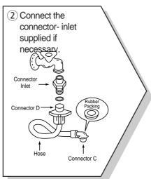
3 Connect the inlet hose adapter to the water inlet of the washer and turn it to be fixed.
