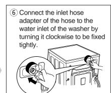
Please check the rubber packing present inside the inlet hose adapter of the hose.
