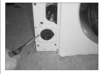
5) Remove the inner drain hose, and remove the drain pump.
