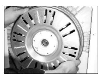
4) Separate the STATOR from the TUB.
