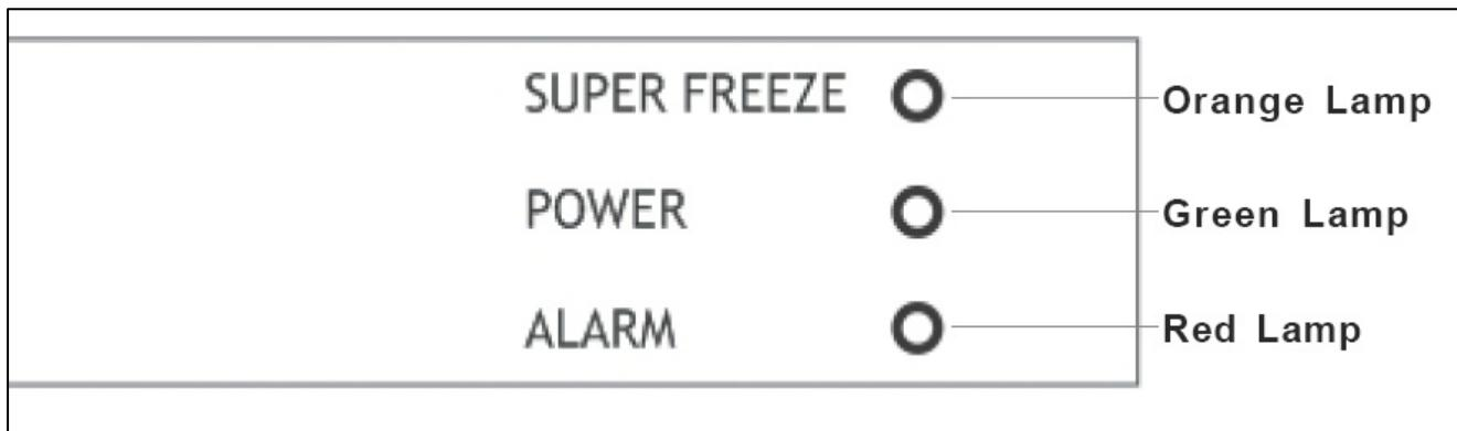
**ORANGE LAMP :** When the “Super Freezing” operation is on (thermostat dial is in SF position), the orange lamp will turn on.
